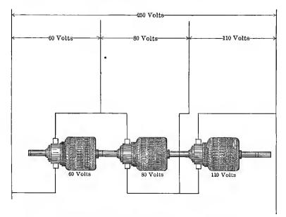
FIG. 150. Diagram showing multi-voltage circuits for shop motors.
